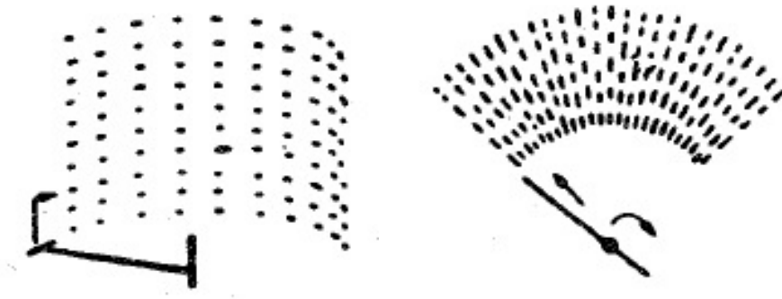
Figure 3.9: Selectors and their movement for a Strowger and for a LME-500 Point Source: Chapuis (1982)
