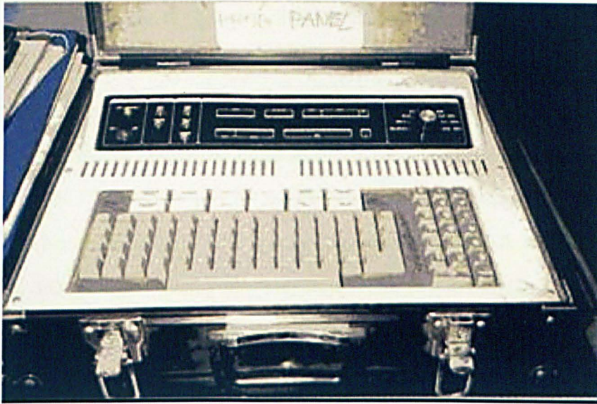
Figure 6.2 - "Suitcase" Programming Device
