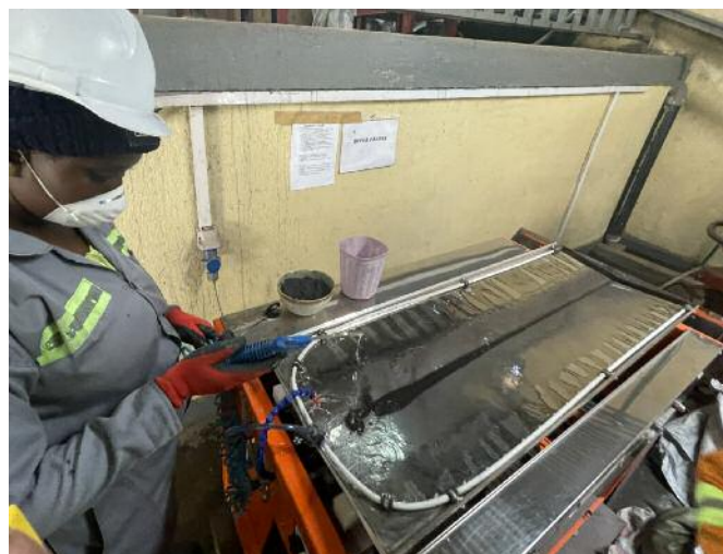
Figure 23: Pilot and lab-scale processing equipment at the metallurgical testwork facilities at the Nyakabingo mine, Rwanda. (left = spirals, right = super-panner)
