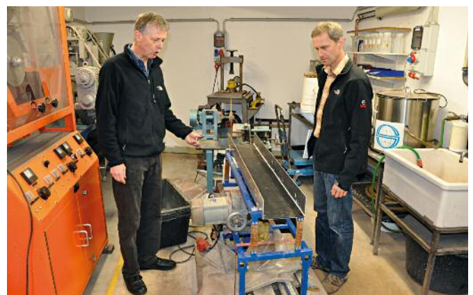
Figure 22: Pilot plant equipment at the Aachen Mining University, Germany used to undertake metallurgical studies for tungsten mining projects. In foreground a laboratory concussion table.
