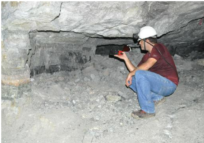
Figure 5: Low-profile room & pillar mining of the "A" orebody at the Bonfim mine, Brazil, showing strong scheelite mineralisation in a narrow band along the top of the skarn layer. With normal light (left), with UV light (right).
