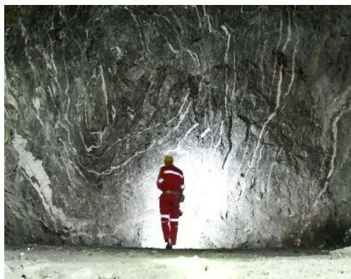
Figure 8: Quartz-scheelite stockwork veining at Mittersill under normal light (above) and UV light (right). This is an exceptionally rich exposure in the mine.
