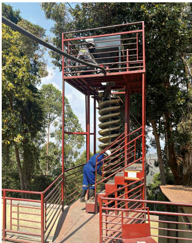
Figure 23: Pilot and lab-scale processing equipment at the metallurgical testwork facilities at the Nyakabingo mine, Rwanda. (left = spirals, right = super-panner)
