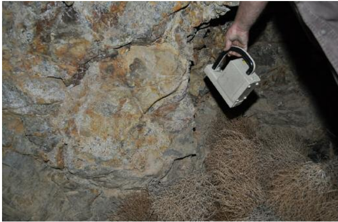
Figure 11: Exploration field work – Breccia-hosted scheelite during night prospection at Darwin in the Californian desert (left flash light, right UV light).
