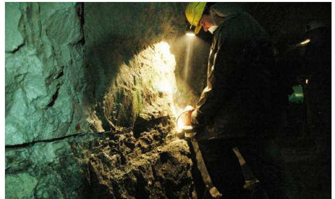
Figure 13: Underground channel sampling at the Rudnik mine, Serbia, testing scheelite mineralisation.
