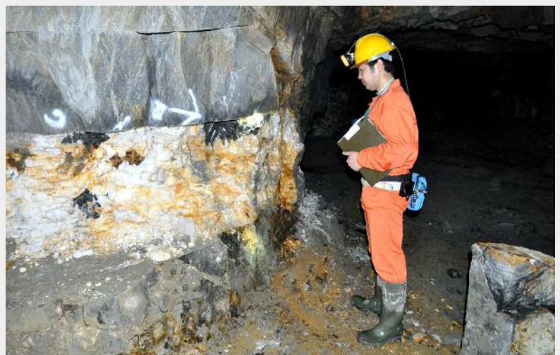
Nuggety wolframite ore at the Panasqueira mine, Portugal. Visual estimates (surface of black wolframite in white quartz) are used to determine the grade. Note: a 2 mm thick “continuous seam” of wolframite would account for a grade higher than the average production grade of the mine.
