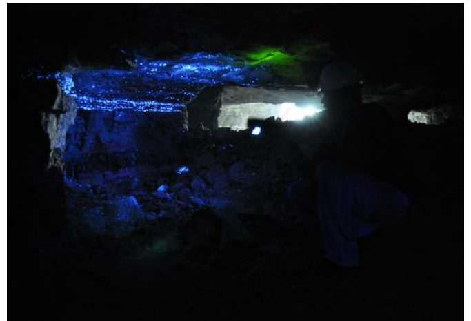
Figure 5: Low-profile room & pillar mining of the "A" orebody at the Bonfim mine, Brazil, showing strong scheelite mineralisation in a narrow band along the top of the skarn layer. With normal light (left), with UV light (right).
