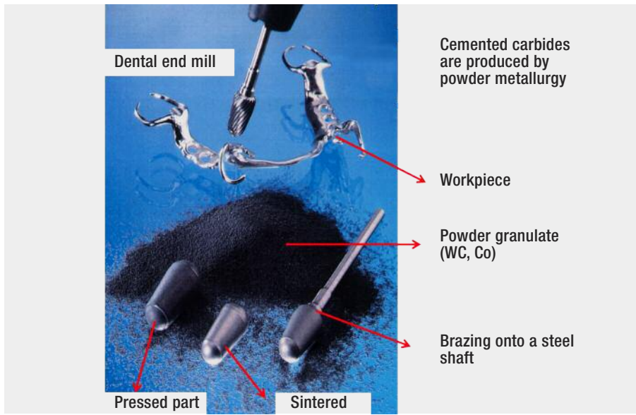
Figure 5: Dental endmill shown in different stages of manufacturing. Note the significant shrinkage which occurred on sintering; during this stage the still porous “green” part is transformed into a dense body of outstanding strength properties; the final shape of the endmill is formed by a post-sinter grinding operation with diamond tools; courtesy of CERATIZIT S.A.
