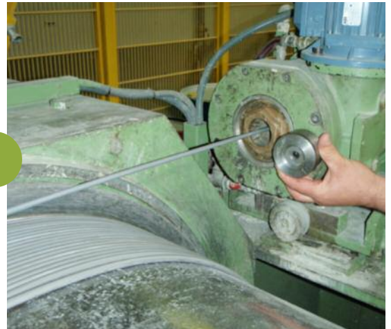
Figure 10: Billions of kilometers of steel and copper wire are annually drawn through cemented carbide dies, or, alternatively, hot rolled over cemented carbide rolls; steel wire is used in reinforcement of concrete, for cable cars, in power lines (together with co-drawn aluminium), cable-stayed bridges, suspension bridges but also as steel cord for car tyres, springs, wheel nuts, bearings, screws, etc.; about 100 kg of steel wire are used in a car.
