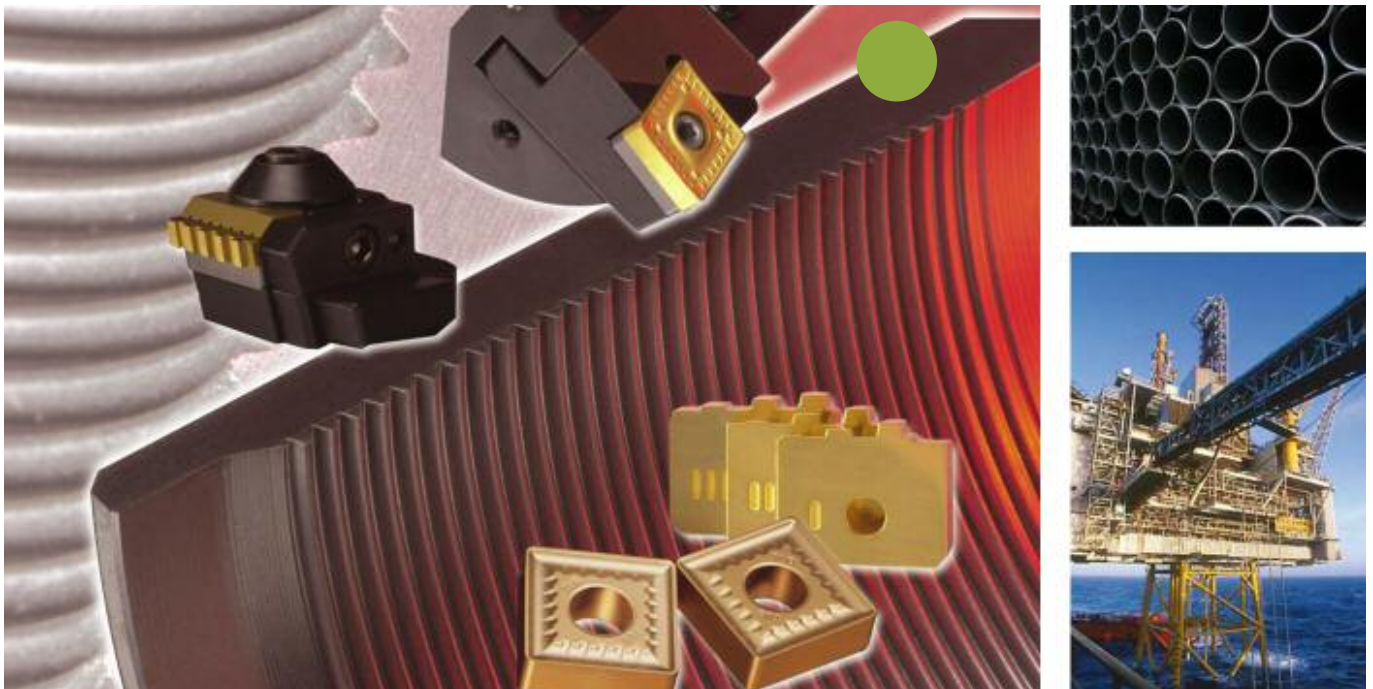
Figure 8: Cemented carbide cutting inserts for threading of tubes; typical grades are coated, fine grained materials (8-12 wt.% Co) with additions of cubic carbides (TiC, TaC); courtesy of CERATIZIT S.A.
