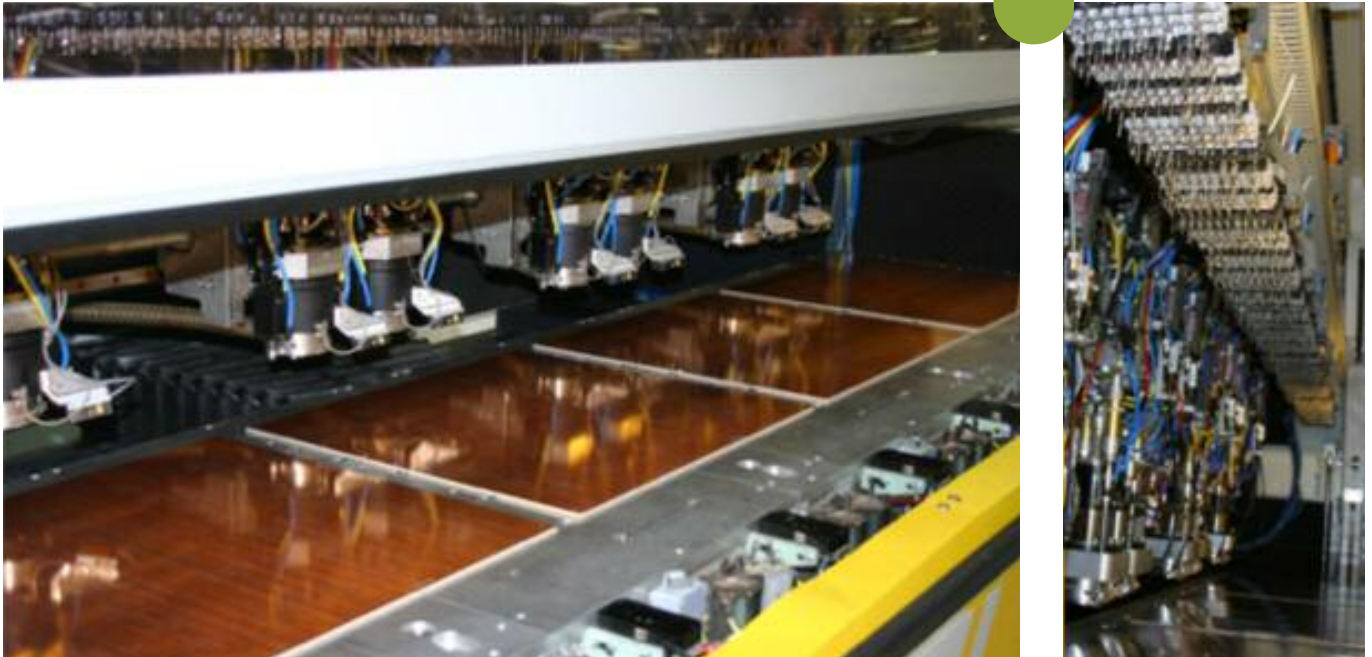
Figure 9: Drilling of printed circuit boards with cemented carbide drills; drill diameters down to 150 \mu\text{m} ; rotating speed up to 300,000 rpm; cemented carbides which are used for this application must have a high hardness (ultrafine grain) and high modulus of elasticity (660 GPa) for precision drilling of very small holes into a copper/glass-fiber reinforced plastic laminate; courtesy of AT&S.
