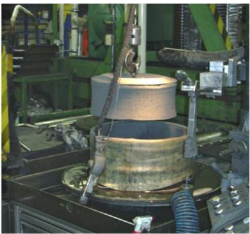
Figure 6: Rod mill roll in the different stages of manufacturing (indirect forming). At first a cylindrical part is formed by cold isostatic pressing (upper image); the part is then formed in the “green” stage by turning with diamond tools (below); after sintering and precision grinding the roll is used worldwide for high-speed finishing blocks in steel works for the hot rolling of steel rod and wire (to the right); typical cemented carbide: extra coarse grain sized WC-Co (6-30 wt %Co, or, alternatively, Co/Ni/Cr); courtesy of CERATIZIT S. A.
