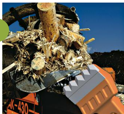
Figure 14: Cemented carbide parts used for wood shredding, but also tree stump grinding, mulching, stone crushing, polymer and textile shredding or chopping of paper roll cores; cemented carbide grades: medium to coarse grained, binder contents between 9–15 wt.%. Courtesy of BETEK.
