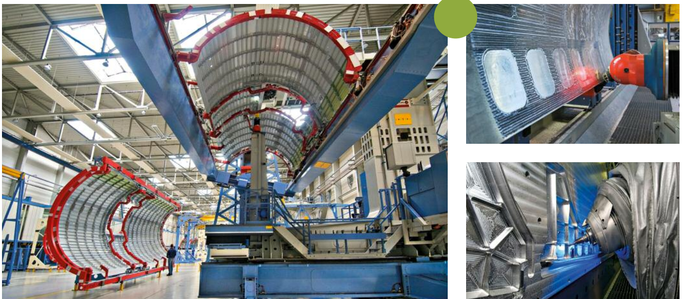
Figure 21: Different stages of manufacturing of a modern airliner; riveting robot for Airbus side shells (left); orbital outline milling robot (top right) and milling of aerostructures at the Augburg plant (bottom right). Courtesy of Premium AEROTEC. Diamond coated cemented carbide tools are used for the drilling of holes into carbon-fiber-reinforced composites; other grades are used for the drilling, milling and turning of high strength steels, aluminium and titanium alloys; about two million holes have to be drilled into the fuselage for the riveting of the CFC-parts with the metallic spars and stringers.
