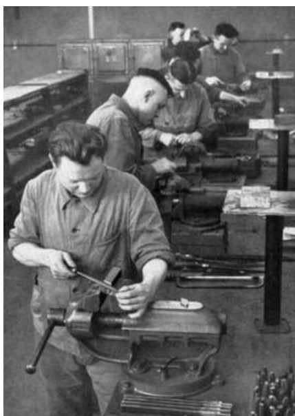
Figure 1: Wire drawing dies with alternating diameter (left); production facility at Widia/ Essen in the early 1930s (right). To produce drawing dies with diamond-like hardness but improved toughness was the driving force for the development of cemented carbides in the 1920s. Field tests were made in the OSRAM factories in 1923 and diamond dies were quickly replaced for the wire drawing of tungsten down to 0.3 mm. In 1925, Friedrich Krupp took over the patent rights and called the new material WIDIA (i.e. like-diamond). Until the mid 1930s, the worldwide production of cemented carbides remained in the range of ten tons per year (statement by Alfried Krupp, chairman of the Krupp AG: “my candy assembly” – referring to the large amounts of steel which was produced at the Krupp AG company in comparison to the new exotic material) [2]. Source: WIDIA-Handbuch, Essen, 1936.
