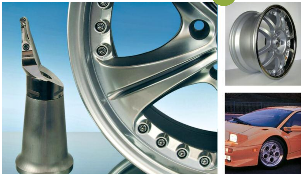
Figure 15: Machining of an aluminium wheel rim with a cemented carbide tool; typical cemented carbide: submicron grain size, WC-Co (5–8 wt.% Co); the PVD-TiAlNcoated tool with an integrated lubricant layer renders the dry machining of the wheel rim and helps reducing manufacturing cost compared to wet machining. Courtesy of CERATIZIT S.A.
