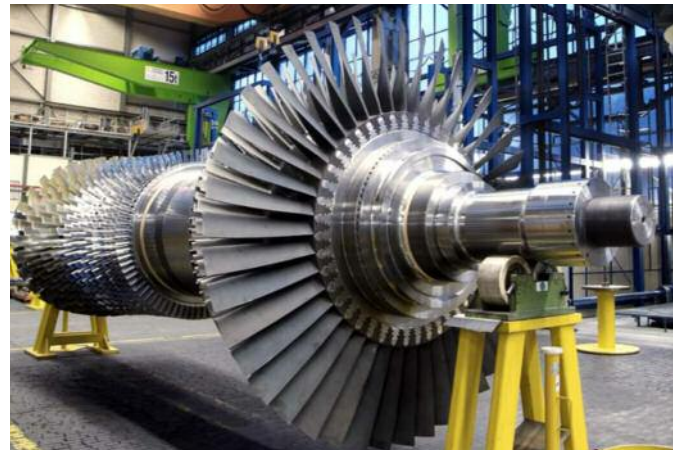
Figure 17: Compressor rotor disk of a gas turbine ready for installation; made of creep resistant steel T505 (left); and turbine rotor (right); © Siemens AG/Martin Adam
