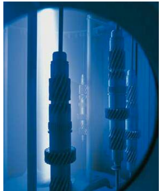
Figure 16: Highly-demanding HSS tools are often PVD or CVD coated to improve productivity in manufacturing. Courtesy of W. Kalss, Oerlikon, Liechtenstein.
