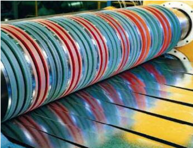
Figure 9: HSS knives are used in large numbers for slitting or transverse cutting of steel tapes, such as tin plate or galvanized heet. Courtesy of M. Gstettner, Böhler Miller Messer und Sägen GmbH, Austria.
