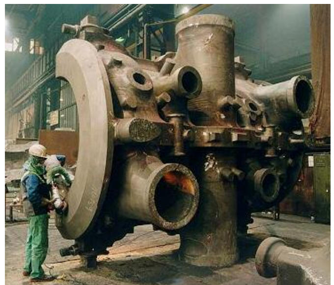
Figure 19: Intermediate pressure inner casing (half), as part of a steam turbine. Weight of the casing is 60 tons. It is made of a martensitic CrMoV-alloyed steel grade containing approx. 1% tungsten (G-X12CrMoWVNbN10-1-1). Courtesy of R. Hanus, Voestalpine Giesserei Linz GmbH.
