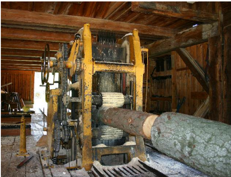
Figure 15: Gang saw for producing wood boards out of a tree trunk; the saws are made of tool steel which is “stellited” (i.e.: the teeth exhibit an overlay of corrosion resistant tungsten-containing stellite). © wikimedia commons/Steindy
