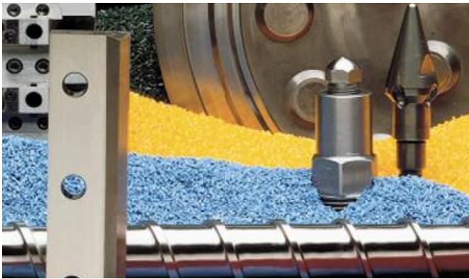
Figure 14: Tool steel for the plastics industry; screw tip and feed screw for injection molding; the demands on the parts have risen due to the increased use of glass fillers; tools are increasingly made by powder metallurgy technology; CPM®. Courtesy of Crucible Materials Corp.
