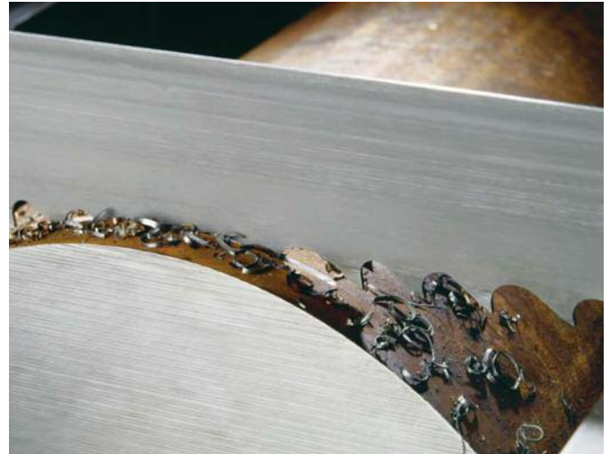
Figure 10: Heavy-duty machining tools are not only used for the machining of steel but also of non-ferrous metals such as nickel-base and titanium alloys; the teeth of the saw blades are made of HSS (M42 bimetal blade). Ccourtesy of K. Rothkehl, Wikus, Germany.
