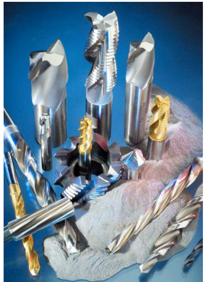
Figure 12: Heavy-duty machining tools produced from powder metallurgy HSS. Segregation-free and homogeneous metal powders of highest purity are processed to homogeneous and segregation-free high speed steels of virtually isotropic properties. Courtesy of Böhler-Edelstahl, Austria.
