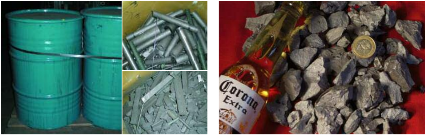
Figure 2: Tungsten is added to the steel melt either as tungsten scrap filled in steel drums (left), or, alternatively, as ferrotungsten (right). Courtesy of Cronimet, Germany.
