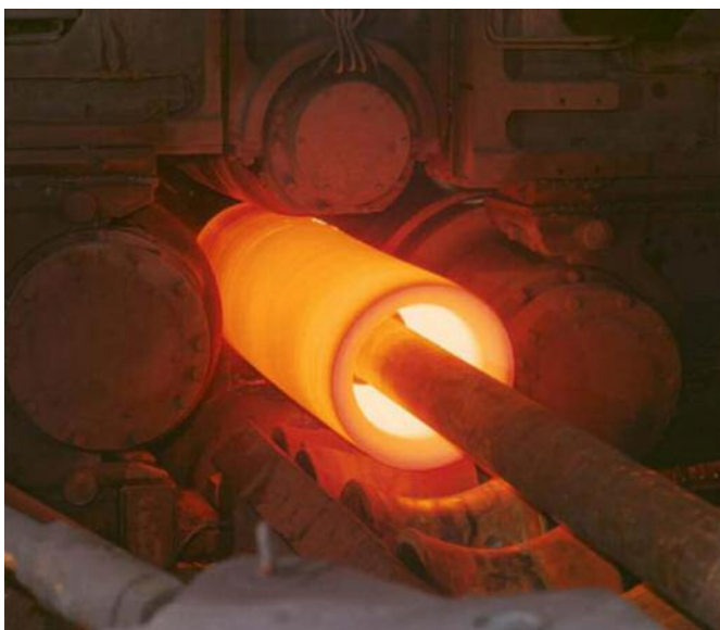
Figure 18: Thick walled seamless pipes of T/P92 materials (X10CrWMoVNb9-2 [max.2% of W]) are produced in a piercing mill according to the Mannesmann process. This material can be used in new modern power plants (T: up to 625°C, pressure: 285 bar) for pressure piping’s, headers and other pressure parts; Courtesy of B. Stroh, V & M Deutschland GmbH, Germany
