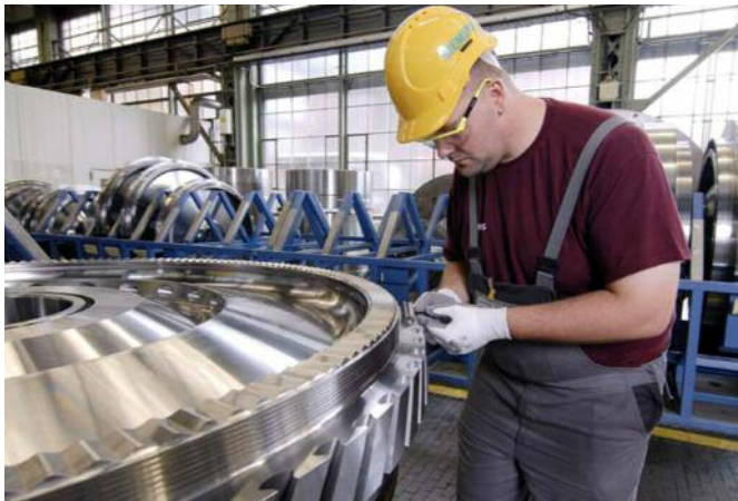
Figure 17: Compressor rotor disk of a gas turbine ready for installation; made of creep resistant steel T505 (left); and turbine rotor (right); © Siemens AG/Martin Adam
