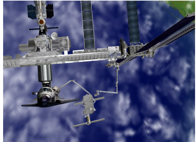
The P6 truss is handed between the station's robotic arm and the shuttle's robotic arm during its installation.
