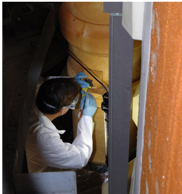
A United Space Alliance external tank technician maps out the cutting area of the LO 2 feed line bracket where BX265 foam insulation and super lightweight ablator, or SLA, cork insulation is to be removed. The BX265 foam insulation was later reapplied without the SLA.
