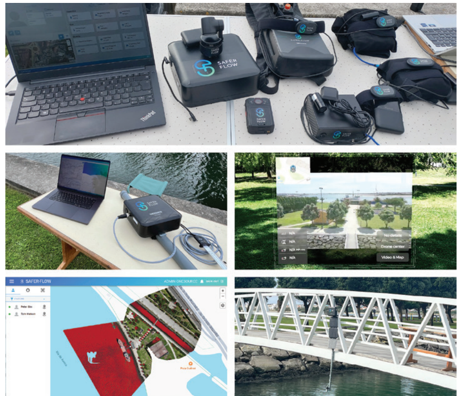
Figure 5: SAFER-FLOW Trial (a: Dashboard of command Control Centre and 5G wearable sensors; b: 5G Water Level Sensor; c: AR point of view with drone video; d: AI/ML Watercourse Detection e: 5G Water Level Sensor showcase)
