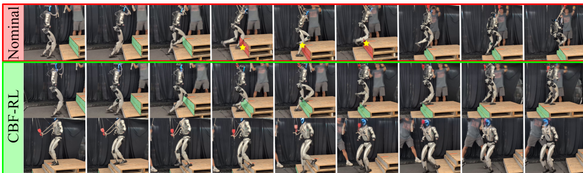
Fig. 6. Snapshots of high stairs of riser height 0.3m. The nominal policy clips its feet against the riser and stumbles, as shown with the red CBF violations while the CBF-RL dual trained policy successfully climbs up and down. The yellow star marks the point the robot’s feet collides with the stair riser.
