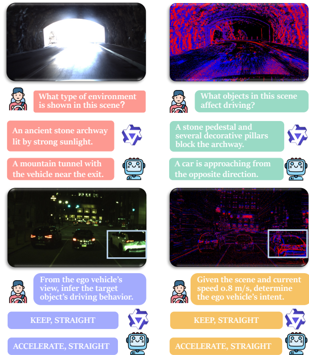
Figure 4. Qualitative results on EventDrive comparing EventDrive -VLM with Qwen. Events remain reliable under low light and motion, improving scene perception, object understanding, motion prediction, and ego intent estimation.
