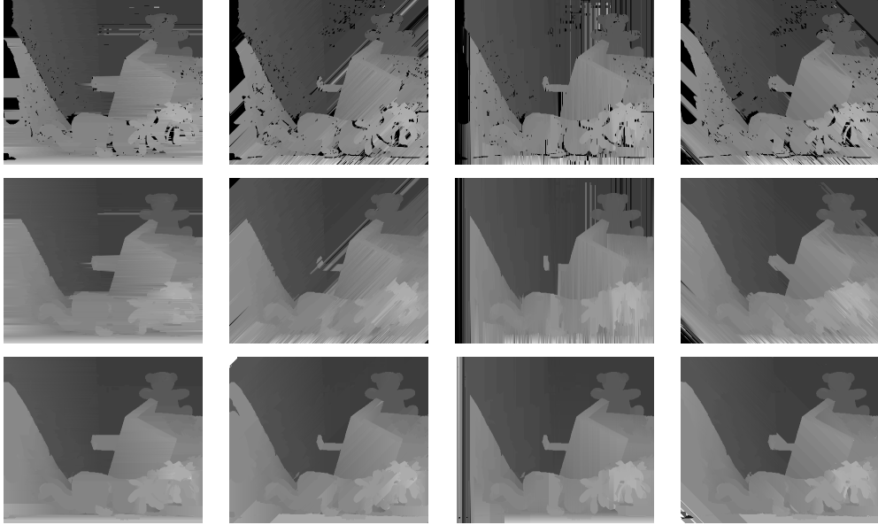
Figure 10: The intermediate results for the “Teddy” image. From the top to the bottom are results of the polynomial regression, results after propagation along the horizontal direction, and results after propagation within regions. From the left to the right are results for line segments where \theta = 0 , \theta = \frac{\pi}{4} , \theta = \frac{\pi}{2} , and \theta = \frac{3\pi}{4} respectively. The results after fusion are shown in Fig. 7.
