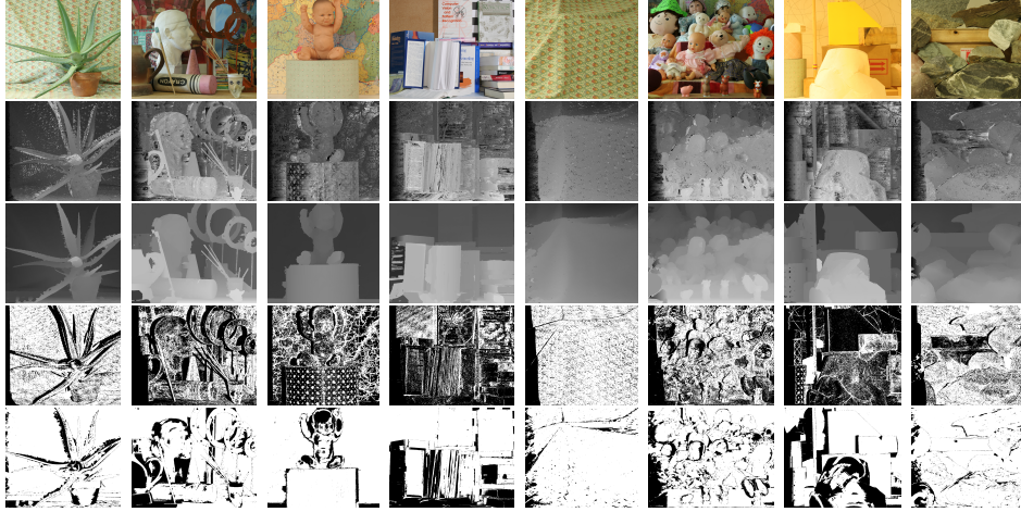
Figure 8: Results on the Middlebury stereo datasets. First row: reference images. Second row: initial disparity map. Third row: our results. Fourth row: error maps of initial disparity map. Last row: error maps of our results.
