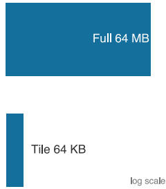
FlashAttention swaps the full attention matrix for small SRAM tiles.
