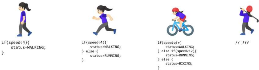
Figure 5.4: Activity Classification Decision Tree: A rule-based decision tree classifies human activity by branching on speed thresholds, with values below 6 km/h mapped to walking, 6 to 20 km/h to running, and above 20 km/h to biking. Real-world edge cases and transitions between activities demand increasingly complex branching logic.
