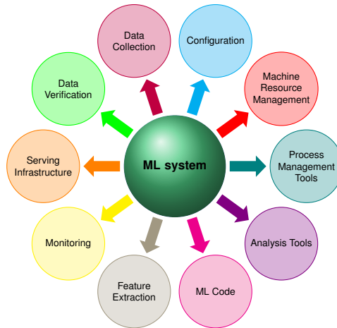
Figure 14.2: Hidden Infrastructure of ML Systems: Most engineering effort in a typical machine learning system concentrates on components surrounding the model itself: data collection, feature engineering, and system configuration rather than the model code. The distribution reveals the operational challenges and potential for technical debt arising from these often-overlooked surrounding components. Source: (Sculley et al. 2015).
