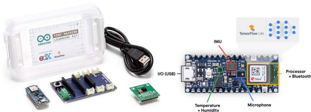
Figure 2.8: TinyML System Scale: Small microcontroller development boards with visible processor chips and pin connectors that enable sensor integration for always-on ML inference under tight memory and power budgets.
