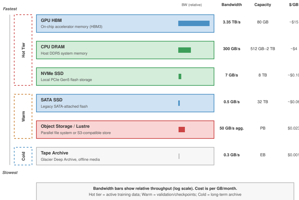
Figure 4.3: ML Storage Hierarchy: Storage tiers grouped into Hot, Warm, and Cold bands, from GPU HBM (terabytes per second, gigabytes of capacity) down to tape archive (sub-gigabyte-per-second bandwidth, very large capacity), with cost per gigabyte changing inversely. The figure adds two tiers beyond the five-level model the prose develops, a legacy SATA SSD tier and the tape archive, to show the full span of the trade-off; the shared object storage and parallel file system tier is filled red because it is the bottleneck that starves a large cluster, the tier whose bandwidth cliff the rest of the chapter works to hide. The figure uses illustrative values to make the bandwidth-vs.-capacity trade-off visible at a glance; the canonical per-tier numbers used throughout this chapter come from table 4.2, which is the source of truth where the figure and the table disagree.
